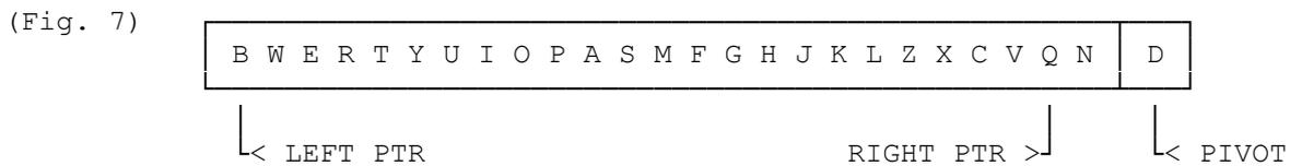
The process is repeated until both pointers cross. The final step of the partitioning is to place the pivot as a separator between the two resulting sub-arrays by swapping it with the item pointed to by LEFT\_PTR:
